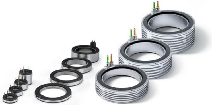
A Tecnotion QTR torque motor kit consists of a rotor containing the magnets and a stator containing the coils. The bigger torque motors are provided with a temperature sensor. A QTL torque motor has optionally a ring with cooling channels wrapped around the stator and four brackets and spacers to fix the rotor and stator in place. In case of the water-cooled motor there are a total of four brackets. Additionally it has integrated temperature sensors. See Figure 2.
