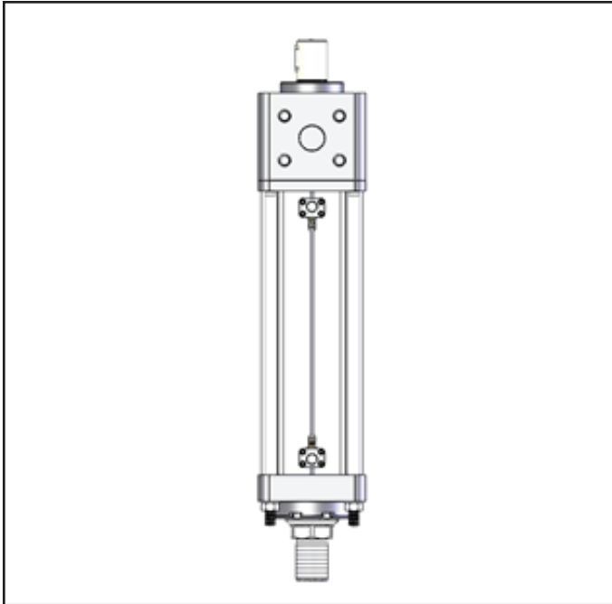
Figure 11b - Vertical Oil Fill Sight Tube and Fill Ports
