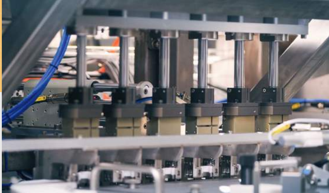
Torque and force sensors enable precise and recordable closing operations, as often required in the pharmaceutical or medical industries.
